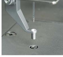
Deactivated lower submergible presser foot – in zero position and in line with the needle plate. Function of compensation for material flexibility is not used and machine works with conventional type of feeding
