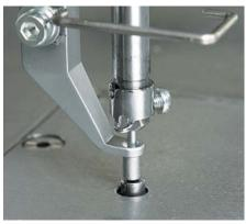
Lower submergible presser foot in its highest position 2.5 mm above the surface of the needle plate performs maximum compensation for material flexibility.
